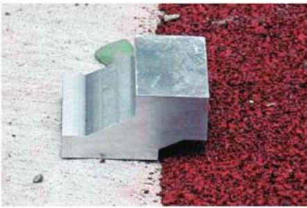
(above) A template is used to measure vertical changes in level.
