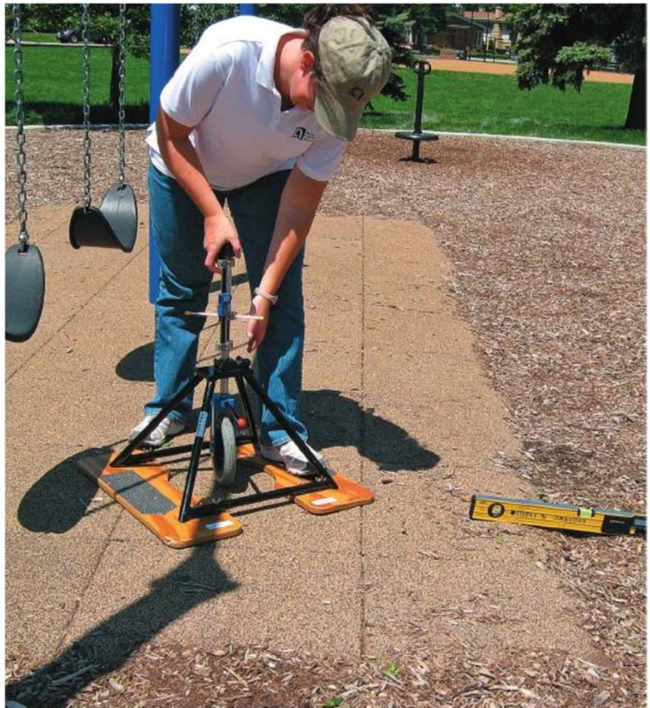
(above) A template is used to measure vertical changes in level.
